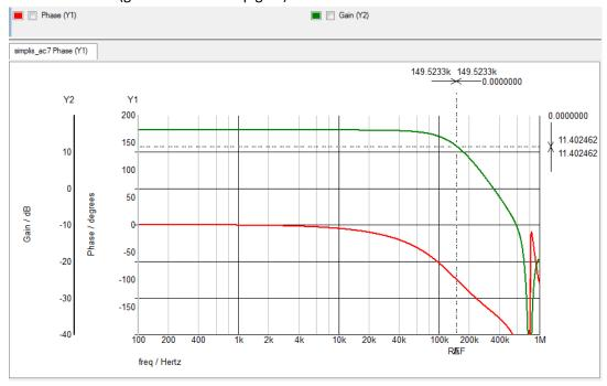
Unstable converter (green = closed loop gain): Gain at 150kHz = 17dB
